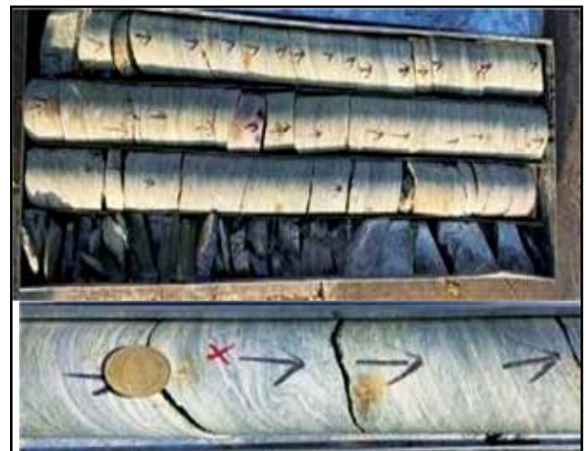
Photo 6.31: Photograph of drill core sample showing evidence of shearing at 163-166 m depth of the BH-APAB-1, Bhadrampalli.
