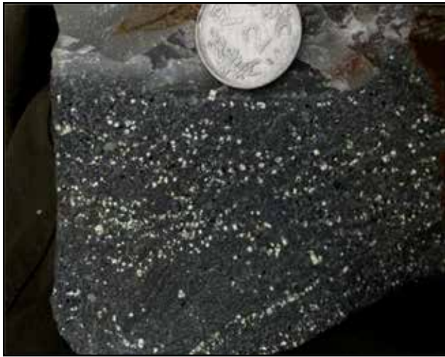
Photo 6.33: Occurrences of arsenopyrite and pyrite from the Venkatpura, Western lode, Gadag schist belt.
