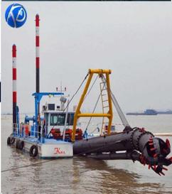
Rotary cutter dredges - Have a cutting tool at the suction inlet to dislodge more consolidated material
