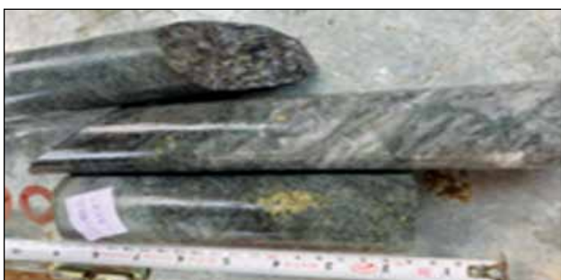
Photo 6.23: Chalcopyrite in BH RJDUBH-02 at 85.20m depth in Gujar-guwara, Dausa district, Rajasthan
