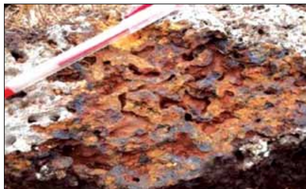
Photo 11.10: Porous concretionary laterite, Champai area, Manipur
