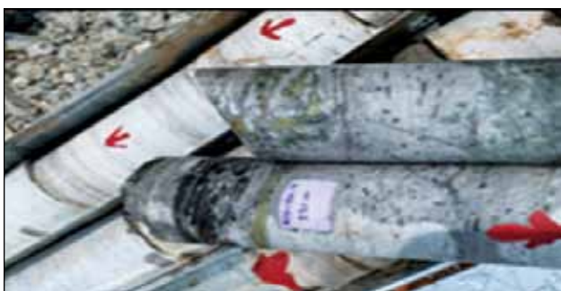
Photo 6.24: Chalcopyrite in BH Rjdubh-04. at 130m depth in Gadarwada-Gujram area, Dausa district, Rajasthan
