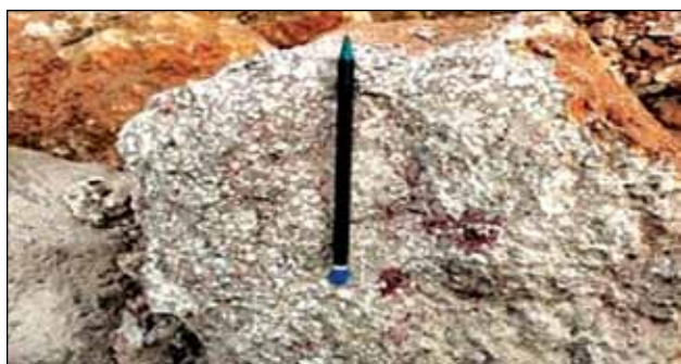
Photo 11.5: Bauxite with pisolitic structure developed over the gneissic rocks of AMGC, near Asimgiri area, Garo Hills, Meghalaya.
