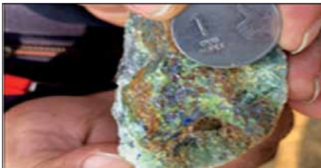
Photo 6.22: Bornite and associated sulphides in core samples of Bhrjdubh-I in Gujar-guwara, Dausa district, Rajasthan
