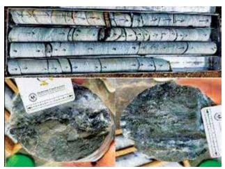
Photo. 6.13. Drilled core of chlorite-sericite schist with sporadic sulphides intersected in APAB-1 in the Bhadrampalli gold prospect.
