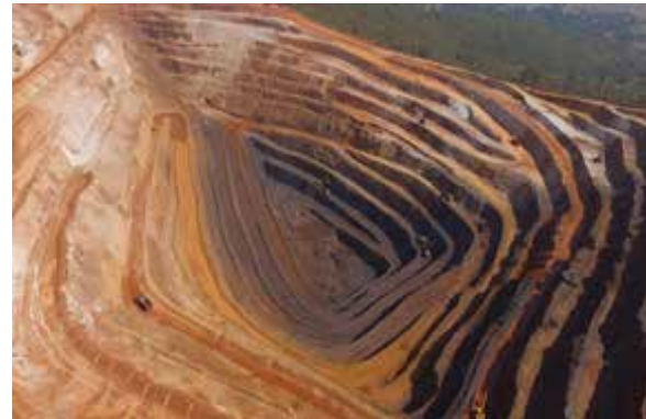
Systematic mining benches in an Iron ore mine in District Sundargarh, Odisha
