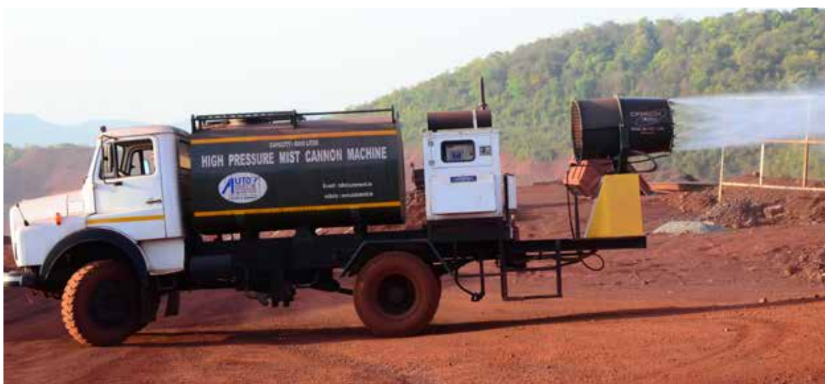
Deployment of advanced mist cannon in mines
