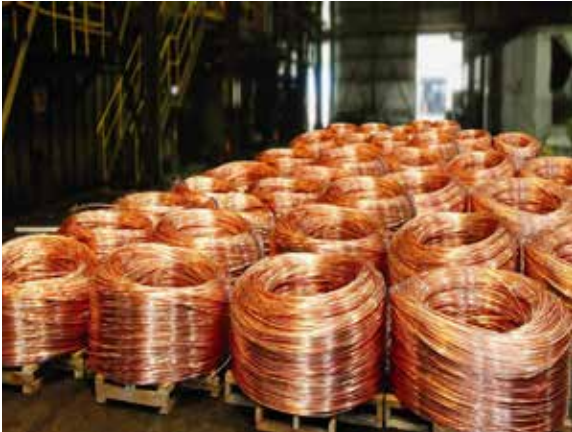
Continuous Cast Copper Wirerod at Taloja Copper Plant
