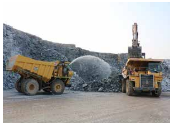
Dust Suppression system at Mine face
