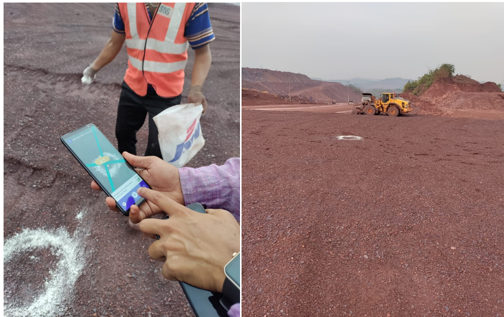
In picture: Generation of sampling points by Augmented Reality based Mobile app.
